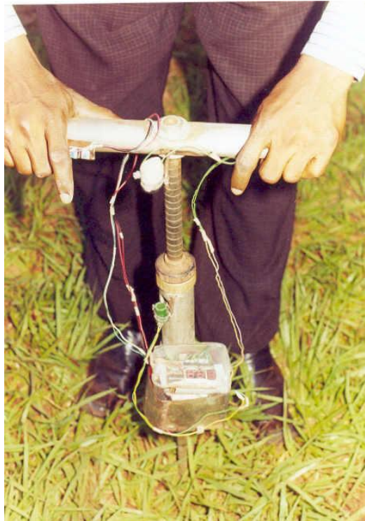
Fig. 6. Penetrometer being tested in measuring soil resistance to penetration.
