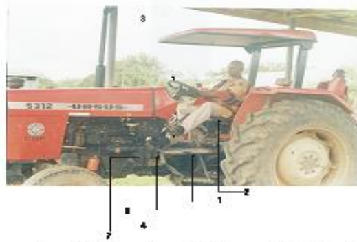
Fig 1(a) Experimental Tractor (1) Frame (2) Seat (3) Steering (4) Foot Pedal (7) Power Transmission Unit (9) Vertical Iron Fiat with Tensile Spring
