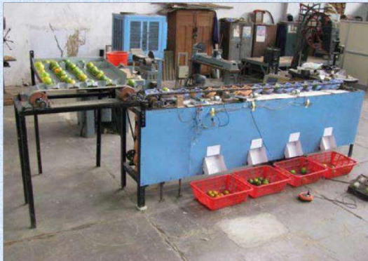
Plate 3.5 Orange grading (weight basis) machine in operation
